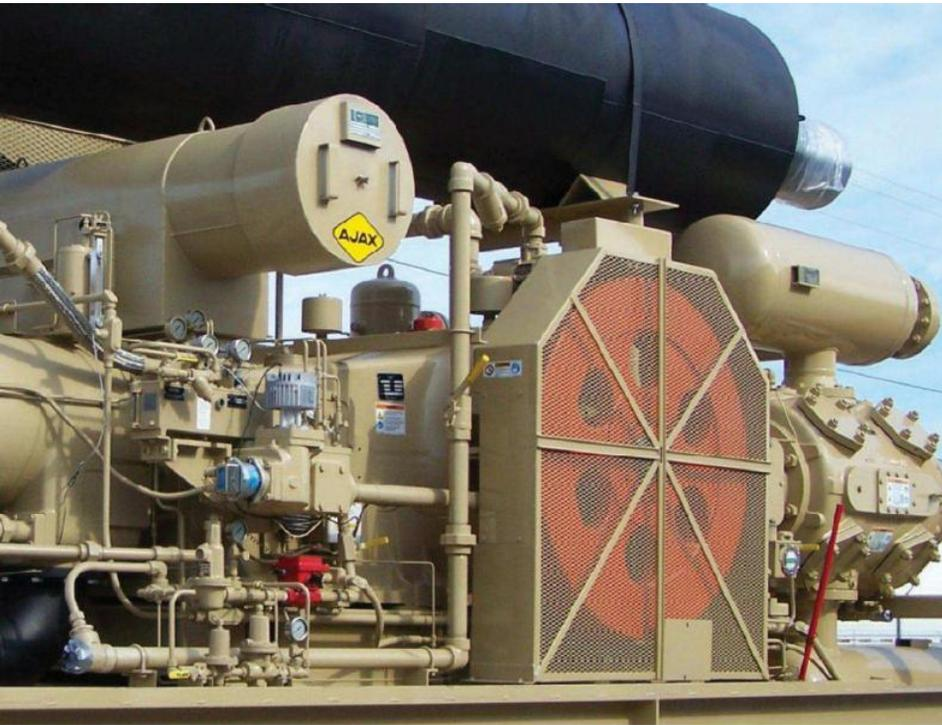
Cooper's initial March test was conducted using a slow-speed integral engine test cell at its corporate headquarters in Houston. The test engine was a standard 2-stroke AJAX 2802 with a 15-in. (381-mm) piston bore, 16-in. (406-mm) power stroke, and a speed range of 360 to 440 rpm.
