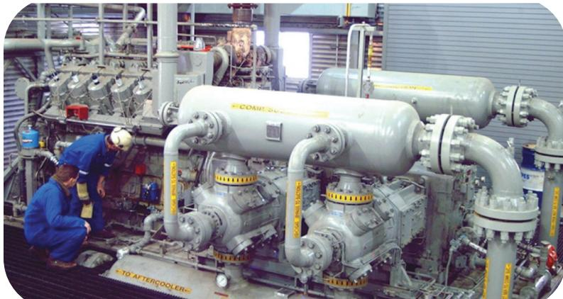
ACI's bypass unloaders are applicable to both new O.E.M. cylinders and reapplied compressor cylinders. Device actuation can be either manual or pneumatic (air or gas).
