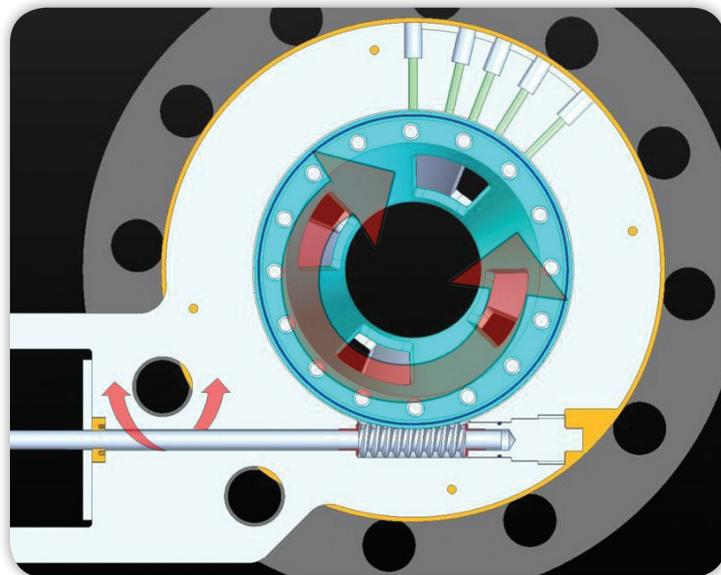
A worm gear rotates the upper ported plate to align its ports relative to ports in the fixed lower ported plate to increase or decrease the DVO Beta ratio.
