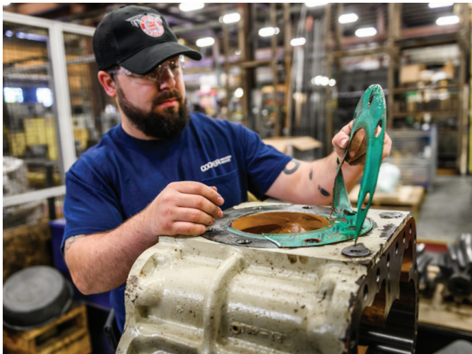
UX Cooper-Bessemer® Oil Pump at Repair Facility
